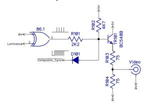
A composite video signal is generated with a sync mixer and video buffer. This is generated alongside the 9" monitor signal, at either 50Hz for PAL or 60Hz for NTSC. The signal has a front and back porch, but no colour burst. When the 12" monitor is selected, composite video is disabled as the 50uS line frequency is not supported. All parts shown above (other than the 74HC86) are optional and can be omitted if composite video output is not required.
