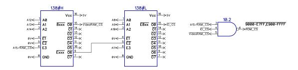
The ROM chip provides ROM in two ranges, from 9000 through to E7FF and E900 through to FFFF. This is implemented here by decoding the video RAM (8000-8FFF) and the IO cut out (E800-E8FF) and selecting the ROM anywhere that is not RAM, video RAM or IO. (Thinking of it that way made the decoding much simpler).
