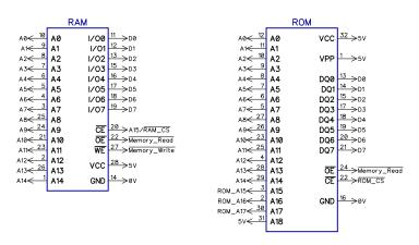
The Mini PET has the full 32K of RAM a PET can support (without paging). This is provided by a single 32K chip, which is decoded simply using the A15 line of the CPU to occupy 0000-7FFF. The ROM is mapped in 32K chunks with 1000-7FFF in the ROM being mapped into the address space as 9000-FFFF. Up to 8 sets of 32K ROM images can be stored in a 27C020 ROM chip and selected using the DIP switches.
