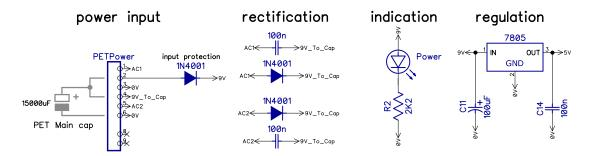
The PET contains a main reservoir capacitor. This is connected to the board via two red wires in the power connector. One feeds 9V DC from the rectifiers to the capacitor, the other takes 9V DC from the capacitor into the circuit. There is a 1N4001 diode as input protection. Previously this was a reverse biased diode which would conduct if there was a negative voltage present. This has been switched to an inline diode to drop the voltage slightly and also protect against negative voltages.
