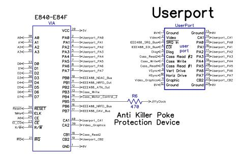
The Jiffy Clock signal is a 60Hz pulse generated by the video circuitry. It was originally used to detect when the screen was not being drawn to allow access to the video RAM without generating 'snow' on the screen. That was no longer required in the later CRTC based PET, or in the Mini PET, and is used purely as a 60Hz timing signal.
