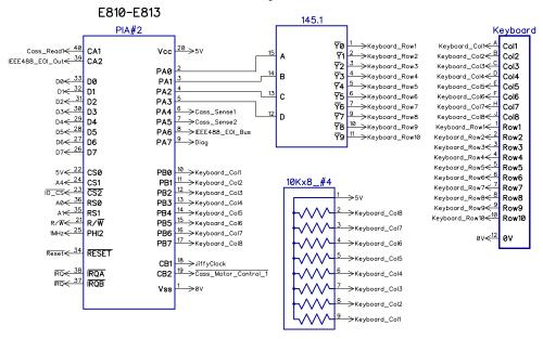
The keyboard is a 10x8 matrix, the rows drive the outputs of a 74LS145 4 to 10 line decoder. The columns are read into the PIA port B, pulled high via a 10K resistor array.
