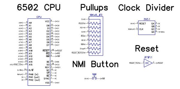
The heart of the Mini PET is the 6502 processor. Here a WDC W65C02S is used. This is a modern version of the NMOS 6502. It is not pin compatible, and the read / write timing differs, so an original chip cannot be used with the Mini PET (nor can anything that would plug into the CPU socket).
