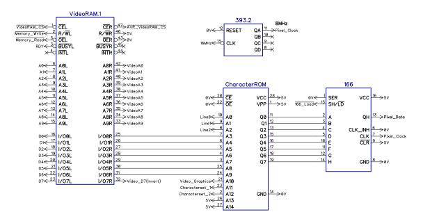
When a character is selected in the character ROM, it's databus contains the bits for one line of pixels that make up the selected character. This is latched into a shift register and clocked out at 8MHz. The pixel data is optionally inverted by an XOR gate controlled by a latch which holds the high bit of character data. The output from the XOR gate is fed via a flip flop which is also clocked at 8MHz, this ensure that all pixels are the same width.
